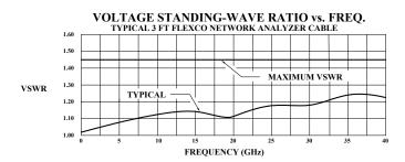
Typical VSWR compared to maximum specification. VSWR remains constant during flexing.
