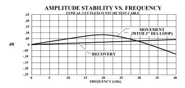
Change in amplitude measures less than 0.10 dB when flexed and exhibits excellent recovery.
