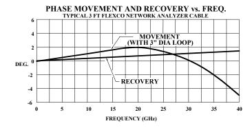
NTC182 VANA Test cables exhibit excellent phase stability when flexed permitting truly accurate measurements.
